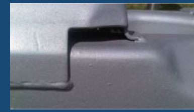
Close Up of Structure and Gap After Welding
