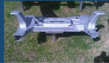
Structure Similar to Rear Suspension Cradle
